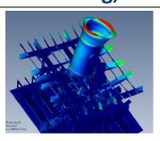
DMS conducted a finite element analysis (FEA) of two crane foundations on a tug with extremely light scantlings. Analysis included detailed modeling of tug structure and crane foundation.
